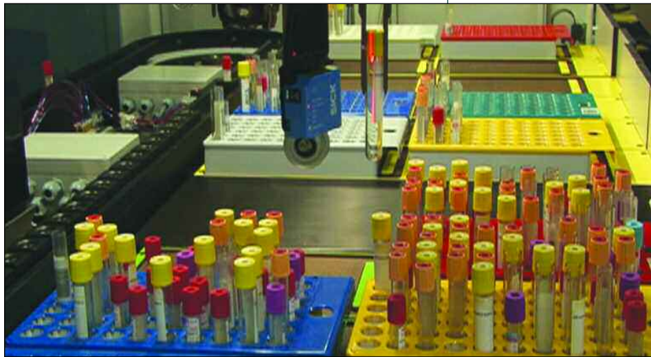
Galil's motion technology maneuvers the robotic arms of NGNY's automated sorter and decapper of clinical lab vials containing human fluids for analysis.
